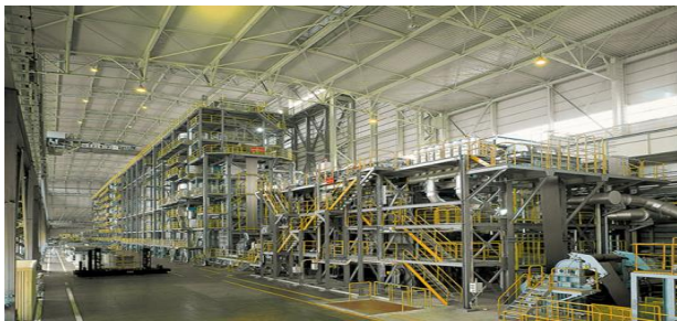
Continuous annealing line for producing steel sheets for use in automobiles
