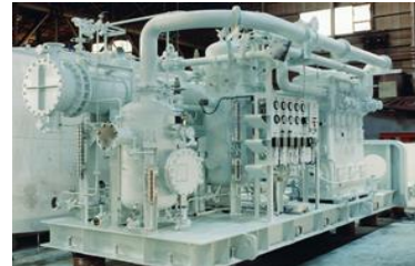
Marine equipment: LPG reliquefaction system
