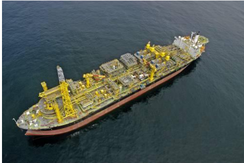
-Floating Production, Storage and Offloading (FPSO) vessel in the Frade Oil Field, Brazil
